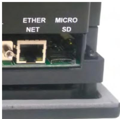
A Micro SD slot is available for data logging purposes. Additional details about using a MicroSD Card for data logging is available in the [Data Logging Overview](#) section. Push against the Micro SD card to eject it from the Touch I/O unit when finished.
