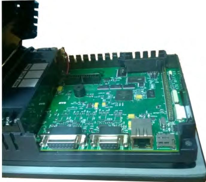
2. The battery is located in the upper-left hand corner as shown in the figure below. Remove the old battery and replace with a new 1/2 AA, 3.6 V Lithium Battery (Part Number: **EZ-BAT**).
