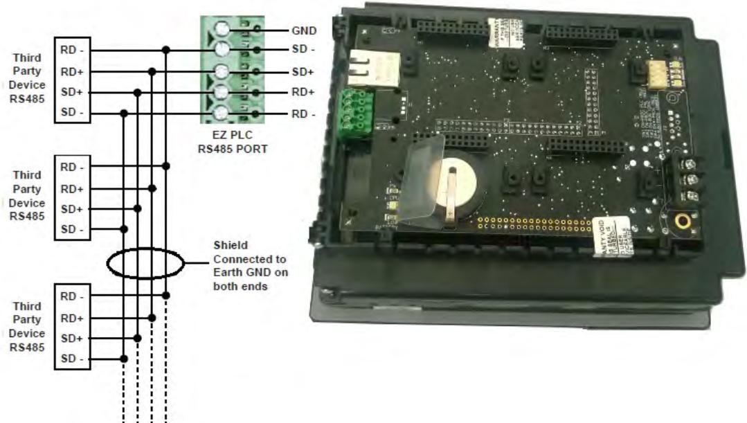
Select models of the EZTouchPLC come with with a RS485 port available on the PLC. This port allows the user to connect to a third party device as outlined above.
