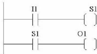
Note: In this example, memory location S1 will be powered when input I1 turns on; you can then use a discrete internal as an input in another rung.
