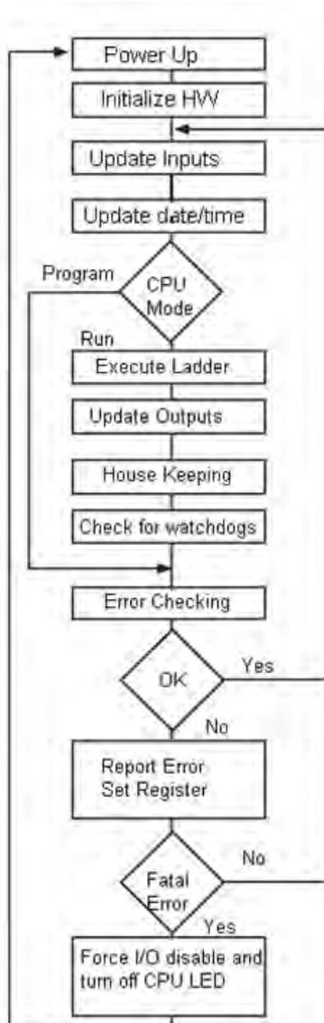
A good understanding of the EZTouchPLC CPU operating sequence will help you achieve the proper control for your equipment or process. The flow chart on the left shows how the CPU controls all aspects of system operation.
