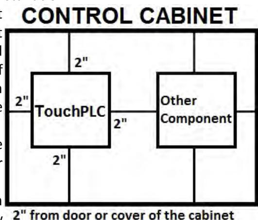
and electromechanical controls. If possible, the electromechanical controls (motors, starters, solenoids, etc.) should be housed separately or at the farthest point when enclosed within the cabinet.
