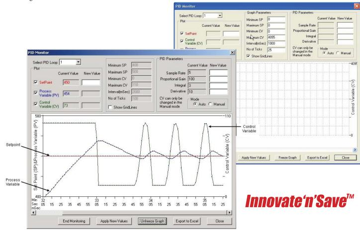
In the illustration above, the Setpoint and Process Variable were set to 450 and are represented by the line running through the middle of the graph. The Minimum SP of 400 is shown at the bottom left and the Maximum Limit of 500 is shown at the top left of the graph. The Control Variable was set to 110 and is represented on the right side of the graph.
