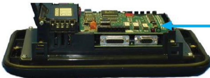
Panel open, showing installed Option Card (Allen-Bradley DH+ is shown)
