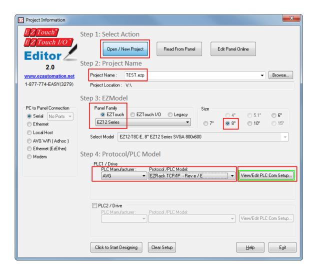
7. Click on "View/Edit PLC Com Setup" and click on "Add" and type in the IP address of the PLC. If you do not remember the IP address, please type in any random numbers, and you can change it later. Click on "OK"
