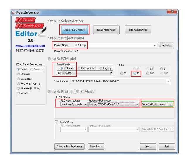
7. Click on "View/Edit PLC Com Setup" and click on "Add/Edit" and type in the IP address of the PLC. If you do not remember the IP address, please type in any random numbers, and you can change it later. Click on "Add PLC Details" and "Close.
