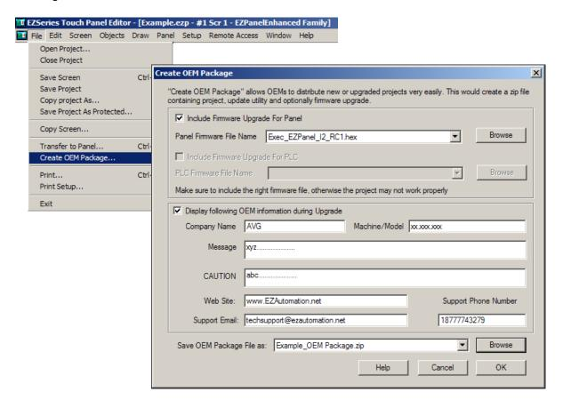
In addition to the project, the packager optionally allows you to include Firmware Upgrade for Panel (and also, optionally, the firmware upgrade for the PLC part if you are working with a TouchPLC).
