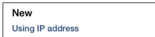
2. A window will appear asking for the Panel Address. Enter the IP address that the panel is located on. The HMI connects on port 10001. The dialogue box therefore shows default port as 10001. Then select *Connect*.
