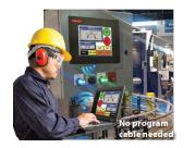
Modular TouchPLC concept that is an all-inone HMI and PLC that can be programmed with a single software, that saves one third of panel space and one third of cost. There are 33 different I/O modules that can be plugged in for an extremely flexible control system design.
